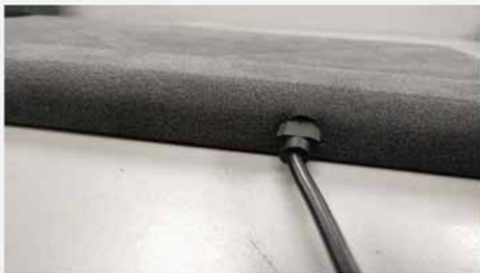
Screenshot 2: Connect MicroUSB cable to the port without opening the Flexi Keyboard.
